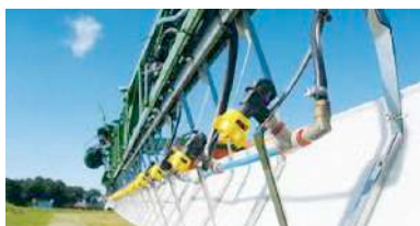
Fig. 14: Crop tilter opens crop for better spray penetration.
