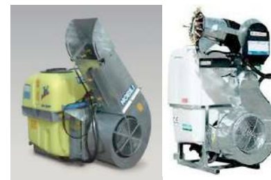
Fig. 13: Cannon sprayer, very vulnerable to drift.
