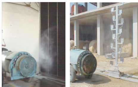
Fig. 28: Equipment to measure the vertical spray distribution.
